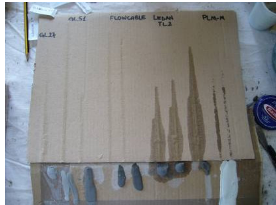
Tests of injection through the tubes in cardboard
