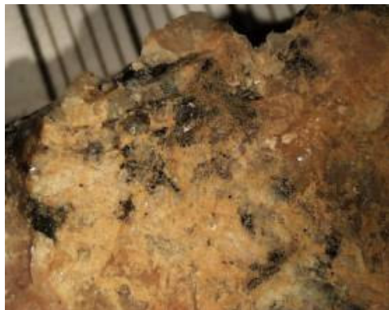
Figure 2: Orange cream deposit in a fissure near the surface of a granite sample coming from the Aswan quarries (1 graduation corresponds to 1 millimetre - photo JM. Vallet)
